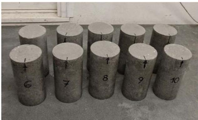
**Fig. 6** Metaconcrete specimens after curing and final polishing.
