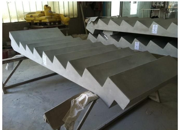
Figure 9. Prefabricated stair ramps / Rampe scale prefabbricate
